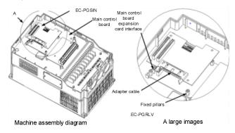
Main control board CN4 slot can stack two different option cards, the specific operation steps is divided into two.
