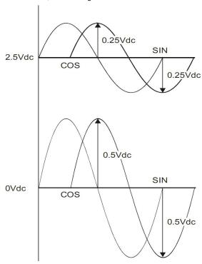
Sigg SinCos encoder signal is as follows, the biggest different with HEIDENHAIN encoders is single ended signal of SinCos signal A, B, for example, A- is not a SinCos signal, it is a signal fixed about 2.5V, and A + is a SinCos signal that offset is 2.5V and amplitude is 0.5V.
