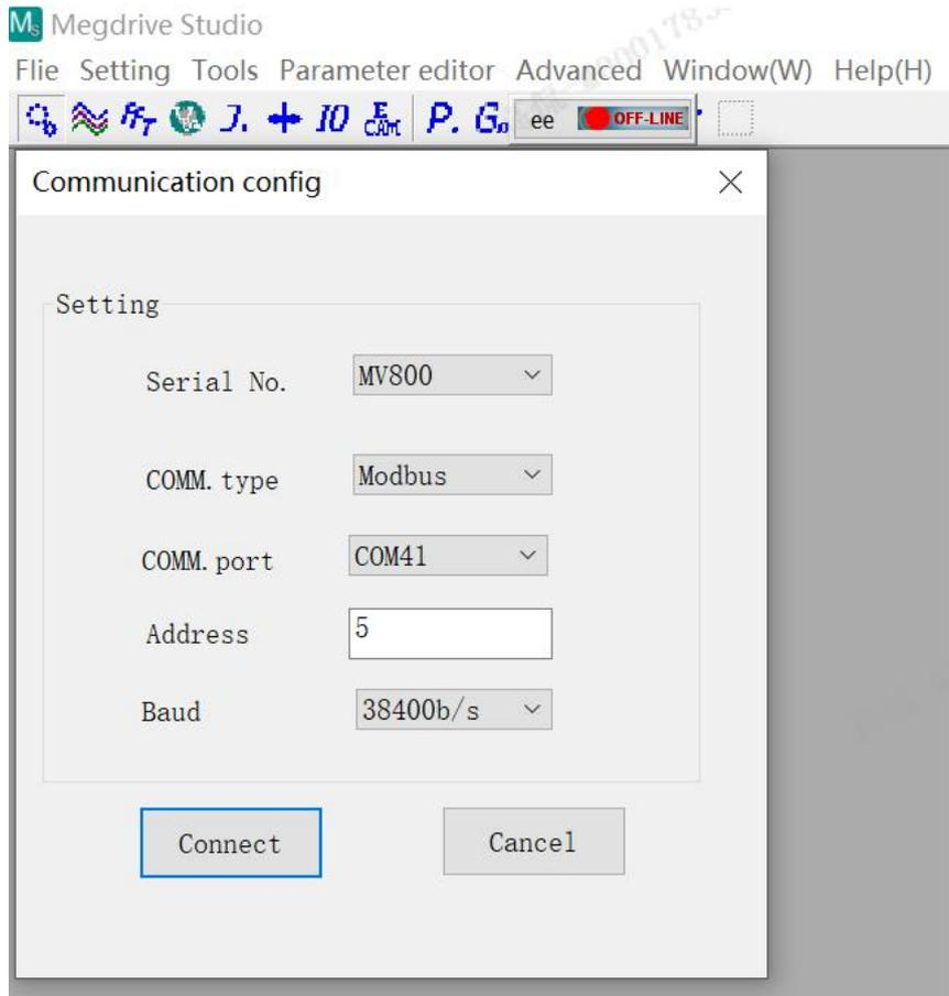
The MV800 model can be configured in the dialog box. The communication type is ModBus. The serial port number is configured according to the specific situation. The communication address and the baud rate are selected by default. After the configuration is completed, click the connection to complete the configuration. If the configuration is successful, the status bar below will light two green lights, as shown in the following figure :
