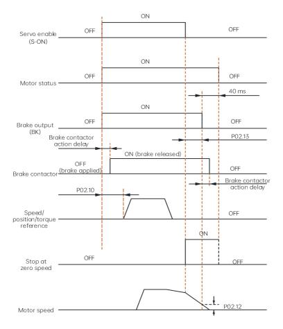
Fig. 6-38 Brake sequence for a rotating motor
