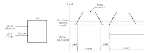
Fig. 6-32 Zero clamp logic
