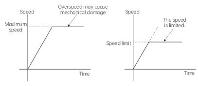
Fig. 6-34 Speed limit in torque control
