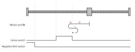
Fig. 6-10 Homing mode 1 motion profile Figure 3
