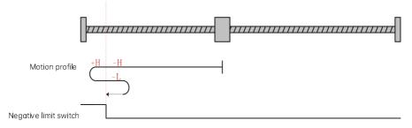
Fig. 6-23 Homing mode 7 motion profile Figure 1
