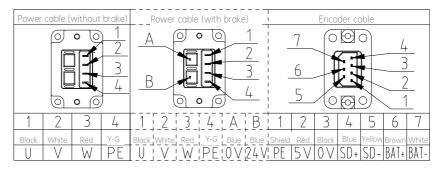
Note: Y-G in the figure means the yellow-green color. The cable color is only for reference. Use the corresponding cable according to its actual definition.
