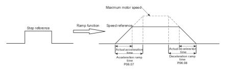
Fig. 6-31 reference ramp function operating logic
