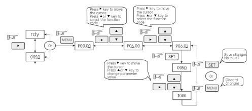
Fig. 5-2 Working status display and parameter setting flowchart
