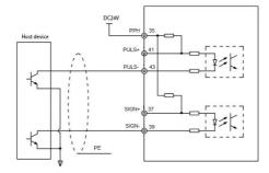
Fig. 4-13 Low-speed pulse reference NPN input wiring diagram
