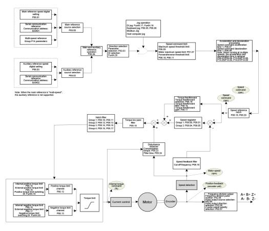
Fig. 6-33 Function block diagram of speed control mode
