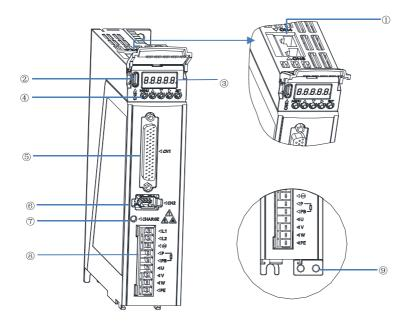
Fig. 1-5 Components of M3-P servo drive (M3-PS2R8A)
