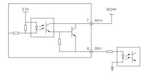
Fig. 4-11 DO terminal PNP (source) output wiring mode
