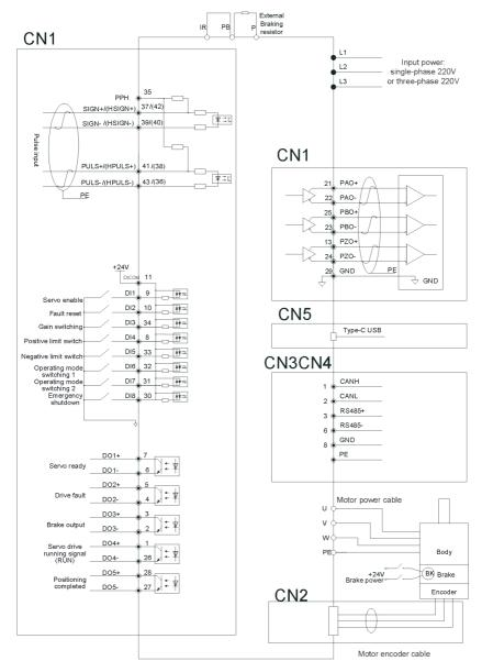
Fig. 6-1 Position control mode wiring
