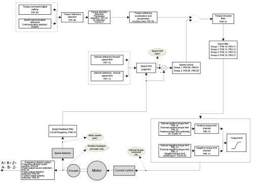
Fig. 6-35 Function block diagram of torque control mode
