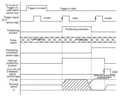
Fig. 6-29 Interrupt positioning sequence diagram
