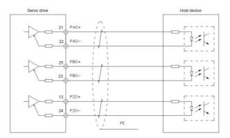
Fig. 4-17 Encoder frequency-division output wiring 2
