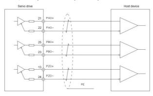
Fig. 4-16 Encoder frequency-division output wiring 1
