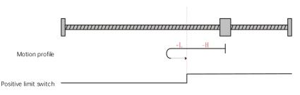
Fig. 6-22 Homing mode 6 motion profile Figure 2
