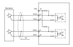
Fig. 4-12 Low-speed pulse reference differential input wiring diagram
