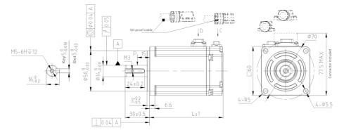
Fig. 2-3 Dimensions for 60 frame medium inertia straight plug economical servo motor (ST4-L series) Table 2-5 Dimensions for 60 frame medium inertia straight plug economical servo motor (ST4-L series)
