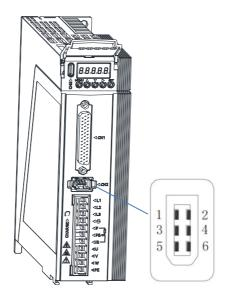
Fig. 4-1 Diagram of servo motor encoder signals
