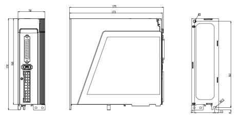
Fig. 2-2 SIZE B servo drive dimensions
