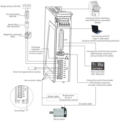
Fig. 3-3 SIZE A single-phase 220 V servo system wiring diagram
