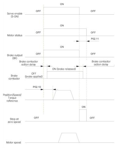
Fig. 6-37 Brake sequence for a motor at standstill
