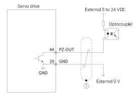
Fig. 4-18 Encoder frequency-division output wiring 3
