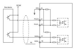
Fig. 4-14 Low-speed pulse reference PNP input wiring diagram
