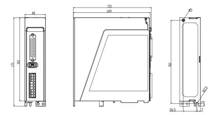
Fig. 2-1 SIZE A servo drive dimensions
