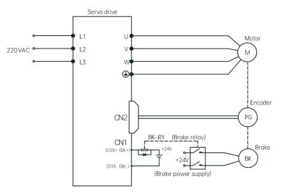
Fig. 6-36 Brake wiring diagram
