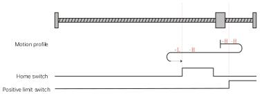
Fig. 6-7 Homing mode 0 motion profile Figure 3
