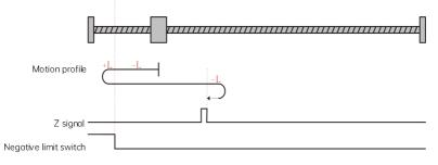
Fig. 6-14 Homing mode 3 motion profile Figure 2
