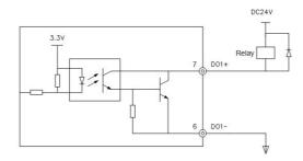
Fig. 4-9 DO terminal and relay wiring mode
