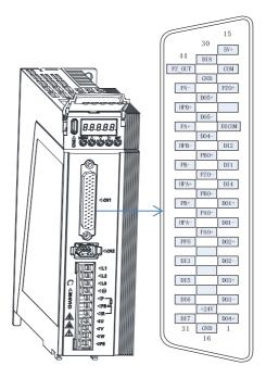
Fig. 4-2 Control signal terminal definition diagram (SIZE A&B)
