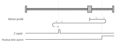
Fig. 6-12 Homing mode 2 motion profile Figure 2
